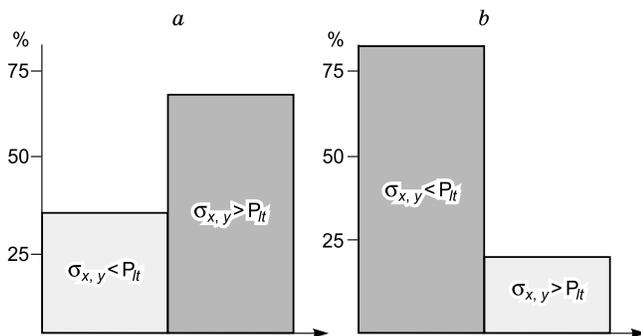
**Fig. 9.** Relative magnitudes of horizontal and vertical stresses ( $P_t$ ) for basement (a) and sediments (b), according to (Markov, 1985).
