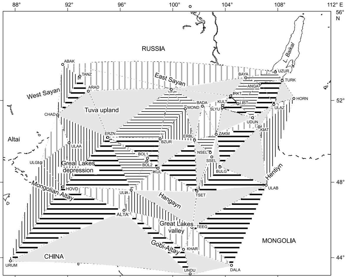
**Fig. 8.** Surface deformation in the Mongolian and Gobi Altay, Sayan, Hangayn, and Baikal, from GPS data. Modified after San'kov et al. (2011), with zones of lateral strain of different magnitudes and directions. Horizontal hatching: lateral extension; vertical hatching: lateral compression; light gray shade: minor change in lateral extent; denser hatching shows higher magnitude of lateral strain; circles mark permanent GPS stations.
