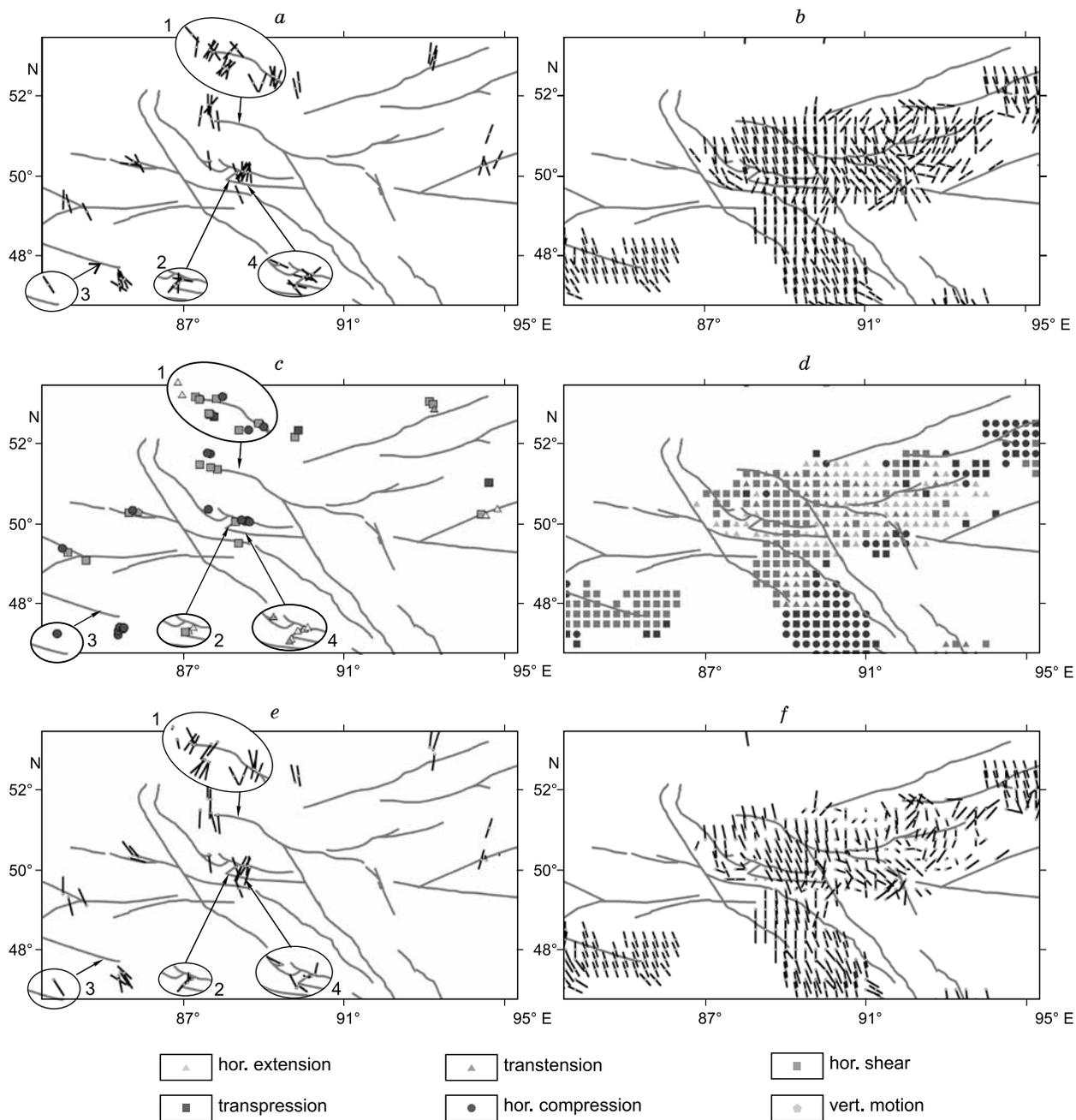
**Fig. 6.** Stress pattern in the Altai mountain area, according to fault slip (*a, c, e*) and earthquake mechanism (*b, d, f*) data ((Delvaux et al., 2013) and (Rebetsky et al., 2012, 2013), respectively). *a, b*, Maximum compression; *c, d*, stress regimes; *e, f*, maximum stress directions. *a, c, d*, Main pattern for Late Pliocene–Early Pleistocene; insets 1, 2, 3: Middle Pleistocene–Holocene; inset 4: Eocene–Miocene.
