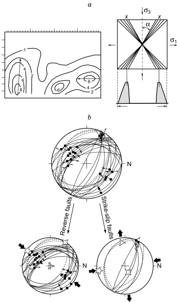
**Fig. 1.** Examples of stress events distinguished by the methods of Nikolaev (*a*) and Angelier (*b*). In the method of Nikolaev (1992), stress states are identified based on maximum density of fracture poles (density contour lines are from 1 to 8 for (*a*) in the left), which have long “tails” along low density gradient (on the right).  $\sigma_3$  is maximum compression. In the method of Angelier (1984), stress events are distinguished according to slip geometry.
