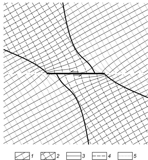
**Fig. 7.** Trajectories of principal stresses and domains of different stress regimes near a left-lateral strike slip (plan view), after (Osokina, 2008). 1, horizontal shear; 2, horizontal compression; 3–5, trajectories of principal stress axes: maximum compression (3), intermediate stress (4), maximum extension (5).
