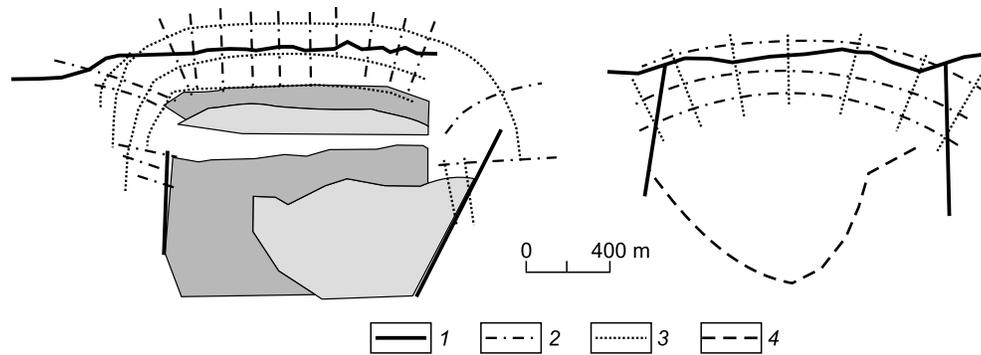
**Fig. 11.** Trajectories of principal paleostresses obtained by Gzovsky (1963) for the Manchabyr anticline (a) and Aksuran syncline (b) within the Bajjansai uplift. 1, faults; 2, trajectories of algebraically minimum principal stress  $\sigma_3$ ; 3, trajectories of algebraically maximum principal stress  $\sigma_1$ ; 4, bottom of Aksuran syncline, simplified after (Gzovsky, 1963).
